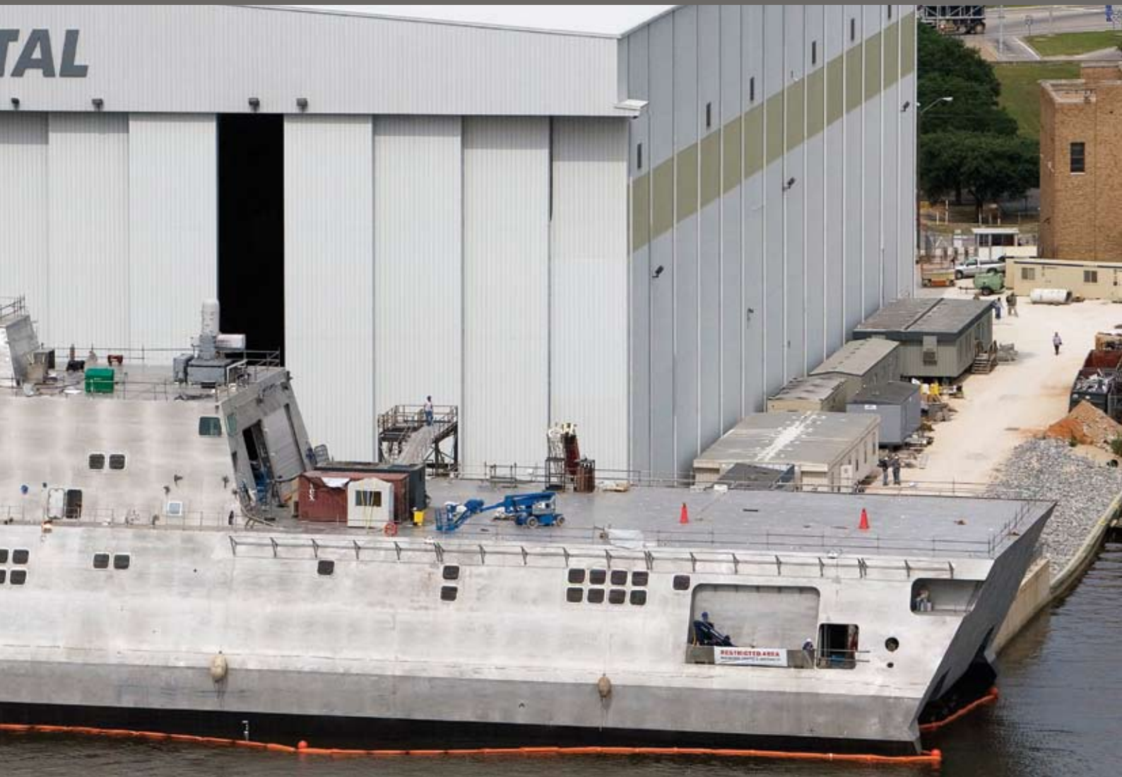
"Independence" is rolled out of the construction hall using sixty-six 100 ton rail trolleys.
