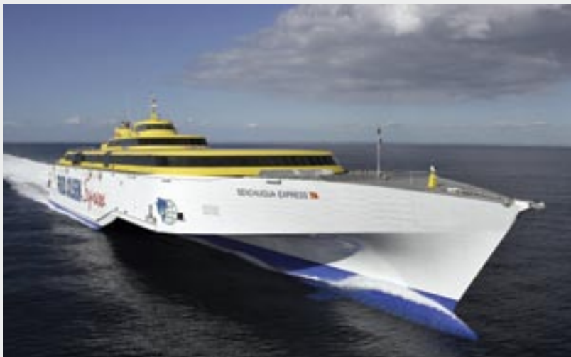
127 metre Vehicle-Passenger Trimaran "Benchijigua Express" at 40 knots – delivered April 2005.
