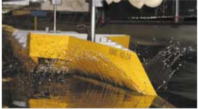
**In 2000 Austal embarked on a comprehensive research and development project aimed at developing a new hull design that would be capable of high speeds in rough seas while at the same time offering unprecedented level of passenger comfort. Analyses identified the trimaran hullform as combining the best attributes of monohull and multi-hull designs to deliver superior seakeeping.**
