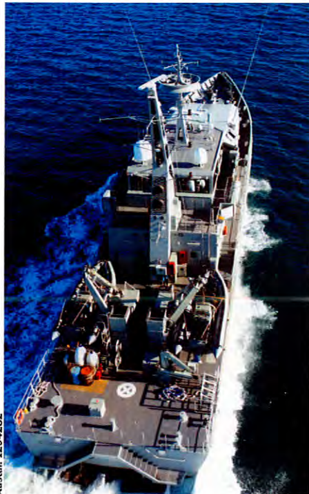
Two 7.2 m RHIBs – shown here on board HMAS Armidale – can be launched and recovered while the mothership is under way, and operate at a distance of 50 n miles.
